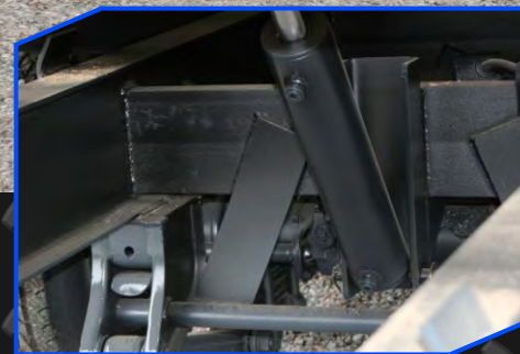
Cushion cylinder controls the deck from slamming when loading or unloading equipment.
