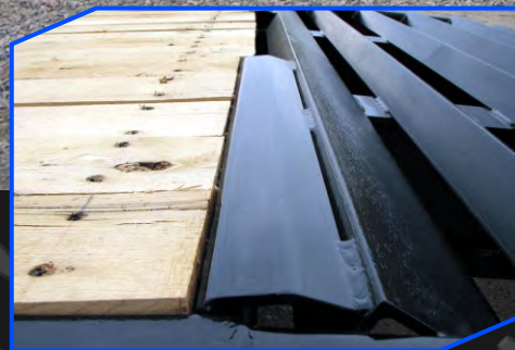
Wood protectors are standard on Big Tow B-series trailers and protect the end of the deck boards.
