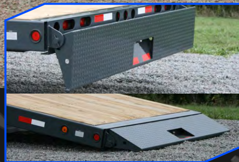
Patented automatic kick-out ramp doubles as under-ride protection.
