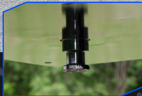
S.A.E. King Pin with smooth approach plate for easy hook-up.
