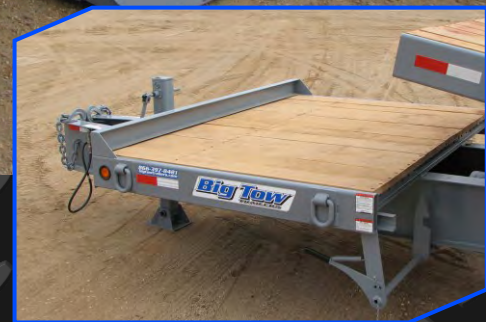
Standard 4-foot stationary deck gives room for longer equipment and makes towing easier.
