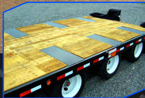
"LP" (Low-Profile) models feature a 10-inch beam, steel over the wheels and a 12-degree beavertail.
