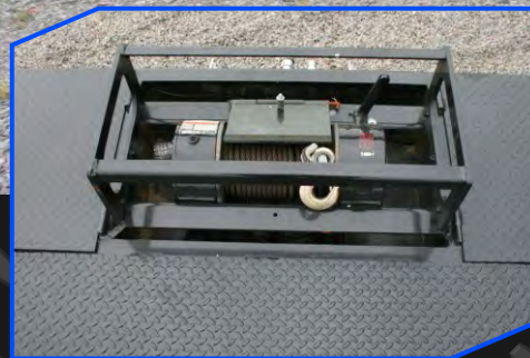
12K hydraulic winch with cable is standard. It is positioned at the front of the 10-foot upper deck of the HT trailer.
