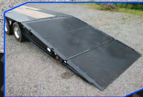
Hydraulic tail creates a low load angle and easy approach. Rear tail section folds under when in transport position.
