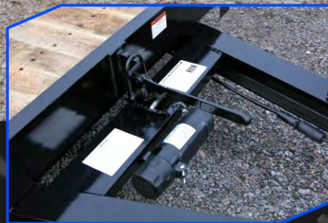
Positive locking (over-center) latch system keeps deck secured to the frame.
