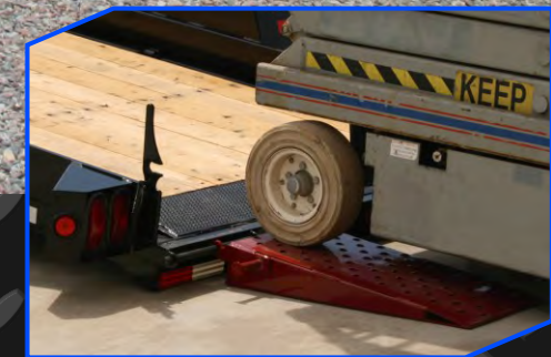
The "SL" (Scissor Lift) option includes ramps to lower the loading incline.
