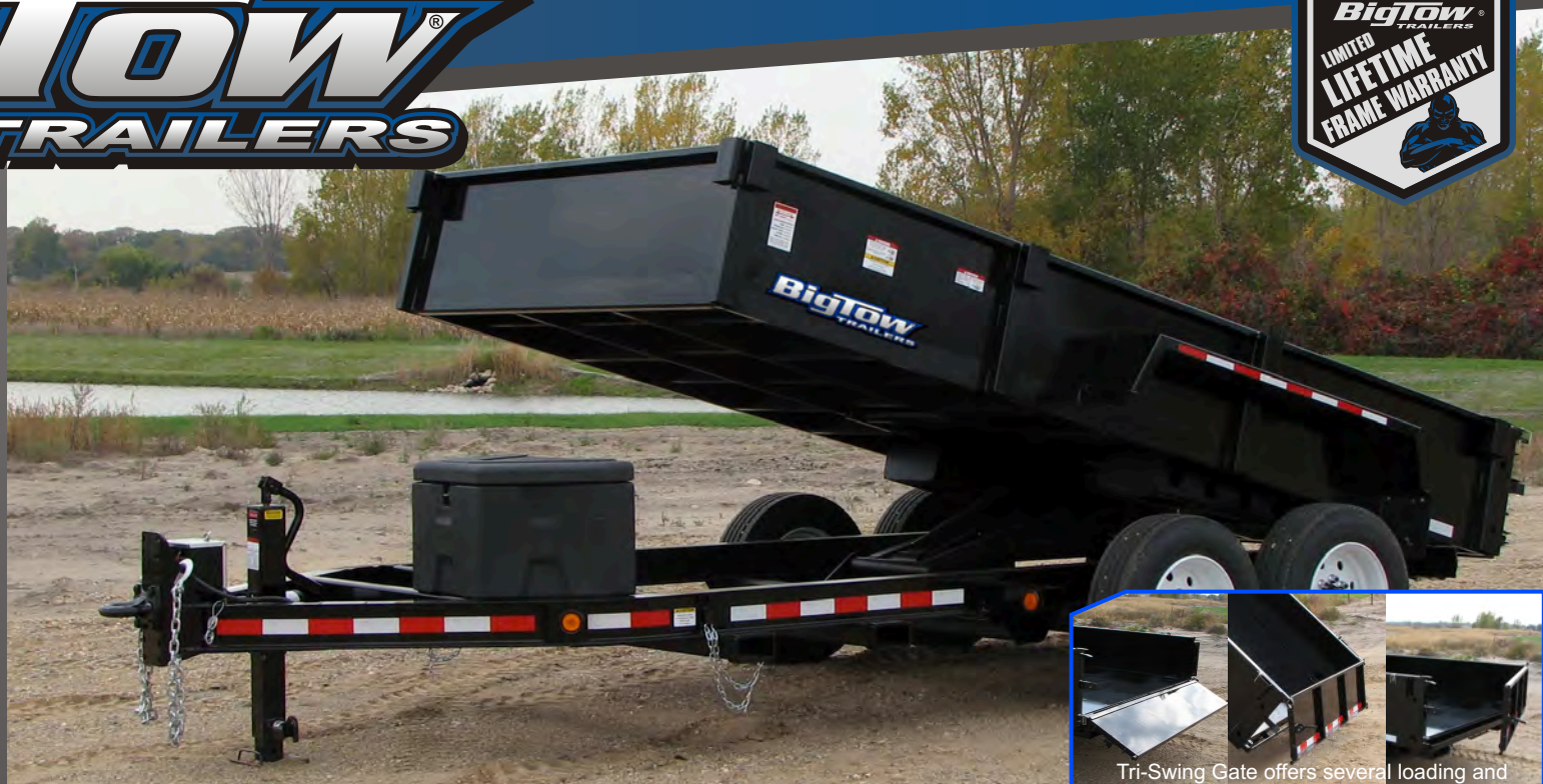
Tri-Swing Gate offers several loading and unloading options.
