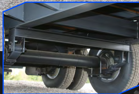
Dexter slipper-spring suspension provides the capacity you need at a budget price.
