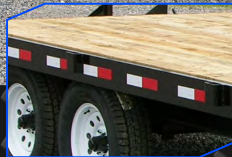
Stake pockets are standard on this model.
