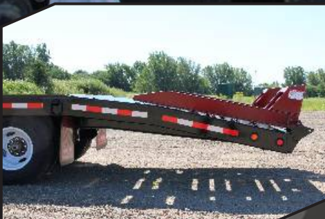
Angle-iron beavertail with 12° to 6° transition to deck.
