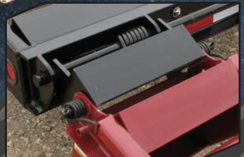
Standard two-way spring assist ramps.
