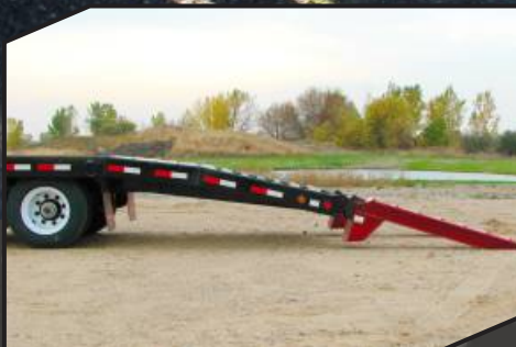
6-foot angle-iron ramps.
