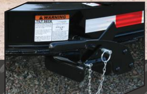
Single deck latch lever with dual latch securement is easy to operate.
